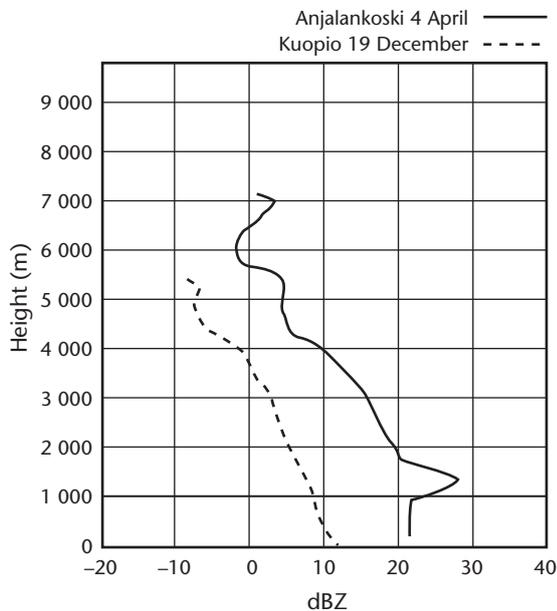
**Figure I.3.9. Two vertical profiles of reflectivity averaged from single polar volumes at ranges of 2–40 km from the radar. The solid line represents rain and the dashed line snowfall (from Koistinen and others, 2003)**
