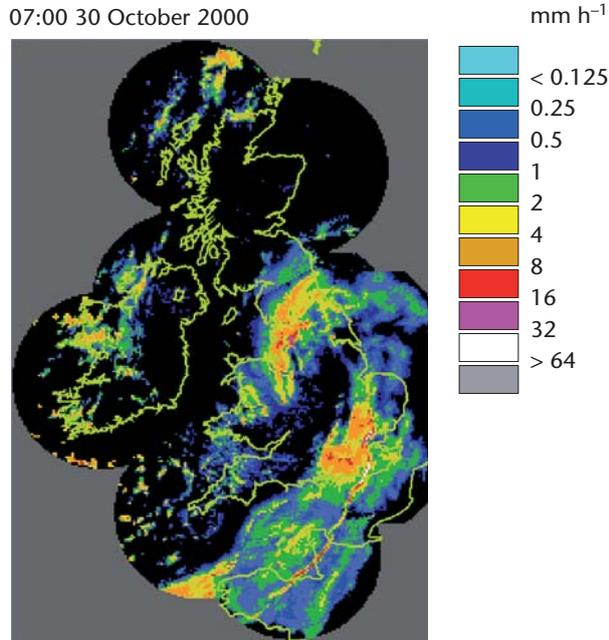
**Figure I.3.10. United Kingdom radar network image comprising radar data from the United Kingdom and Ireland at 0700 UTC on 30 October 2000. The different colours represent different rainfall rates in mm h<sup>-1</sup> as shown. The coastline is shown.**
