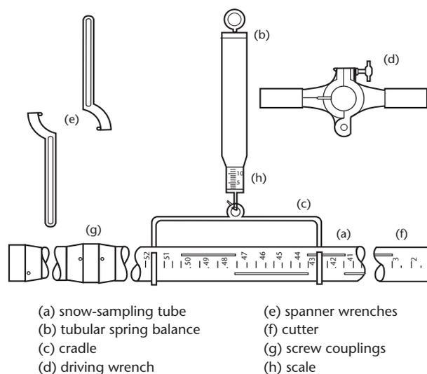
Figure I.3.8. Snow-sampling equipment
