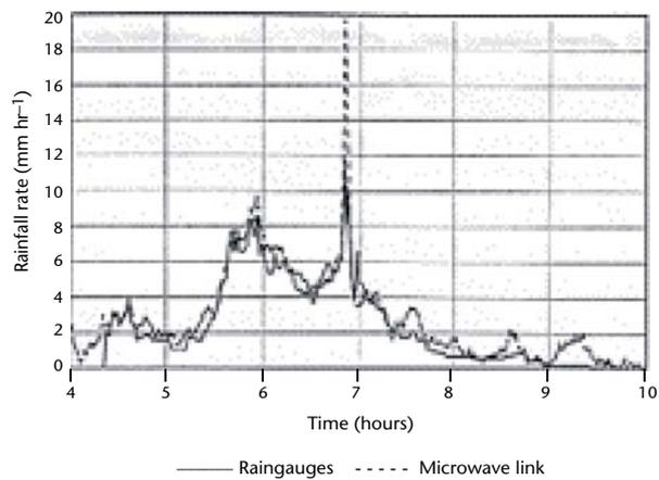
**Figure I.3.11. Time series of path-integrated rainfall estimates from raingauges (solid line) and dual frequency microwave link (dashed line) attenuation measurements over north-west England on 10 February 2000**
